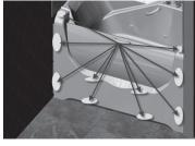
· Press firmly on the following areas to secure the panel.
