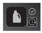
A request for lower-tub maintenance on the display can be postponed by pressing the selection button.
