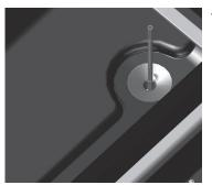
Lift and remove the drainage component from the basin drain.
