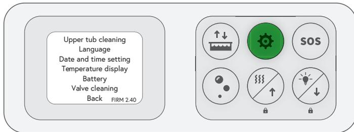
2. Using the arrows, select "Valve cleaning" and press the selection button
