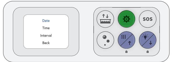
5. Using the arrows and the selection button, select the date on which you want to start the cleaning sequence.
